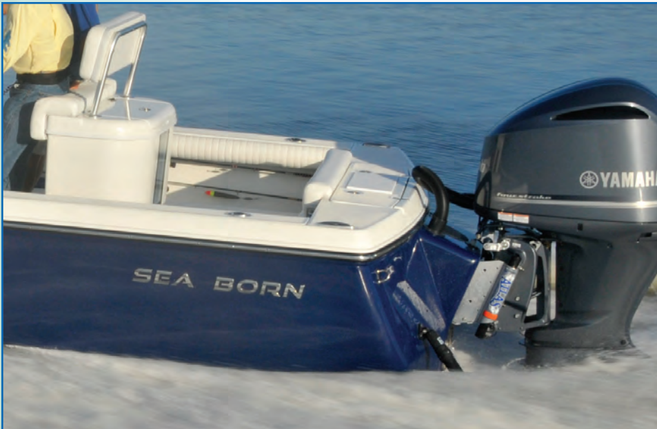
Sportfish Style Fully Enclosed Transom with Molded Engine Bracket
