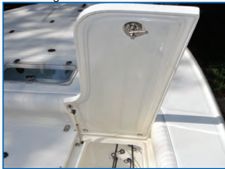
Lids Finished both sides w/ Gas Shocks
