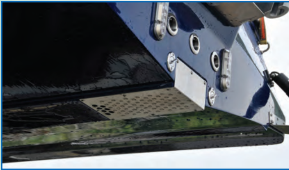
Molded Sea Chest with Hi Speed SS Strainer
