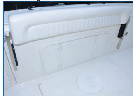
Large Transom Hatch to access Pumps
